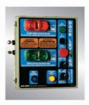
The ultimate in dock safety and performance. A single control station for both Hydraulic Dock Leveler and TL85 Hydraulic Vehicle Restraint. Leveler operation is prevented until truck restraint is secured for operator safety. Standard when ordered in combination with FH Hydraulic Dock Leveler and the TL85 Hydraulic Vehicle Restraint.
